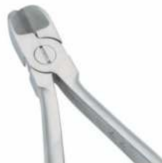
CG-1449 Hard wire cutter, easily cuts any size arch wire or pin. The inserted tips ensure precision cutting and perfect tip alignment. Minimum Cutting Capacity: .012"(.30mm) Maximum Cutting Capacity: arch wires up to .021"x.025"(.55mmx.64mm)
