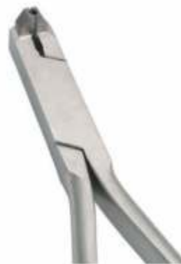
CG-1444 1-Distal End Cutter Flush Cut This instrument cut wires close to the buccal tube and safely holds the distal end. The tungsten Carbide insert ensure precision cutting, long wear and unsurpassed cutting performances. Maximum Cutting Capacity. arch wires up to .021"x.025"(.55mx.64mm)
